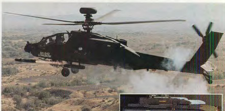
Among the ordnance carried by the AH-64D Longbow Apache are the AGM-114 Hellfire AT missile (outboard on wing, inset) and the AGM-65 Maverick TV guided missile, either of which can service their appropriate targets with pinpoint accuracy.
